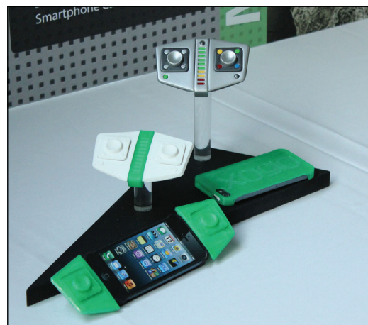
PHOTO BY PETER DAVEY A mobile device game controller design called the Zogo, the thesis project of Humber industrial design student Ian Cameron.
